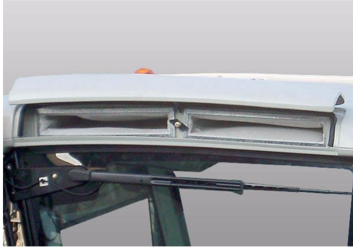
Figure 12 Showing Position Of The External Cab Filters
