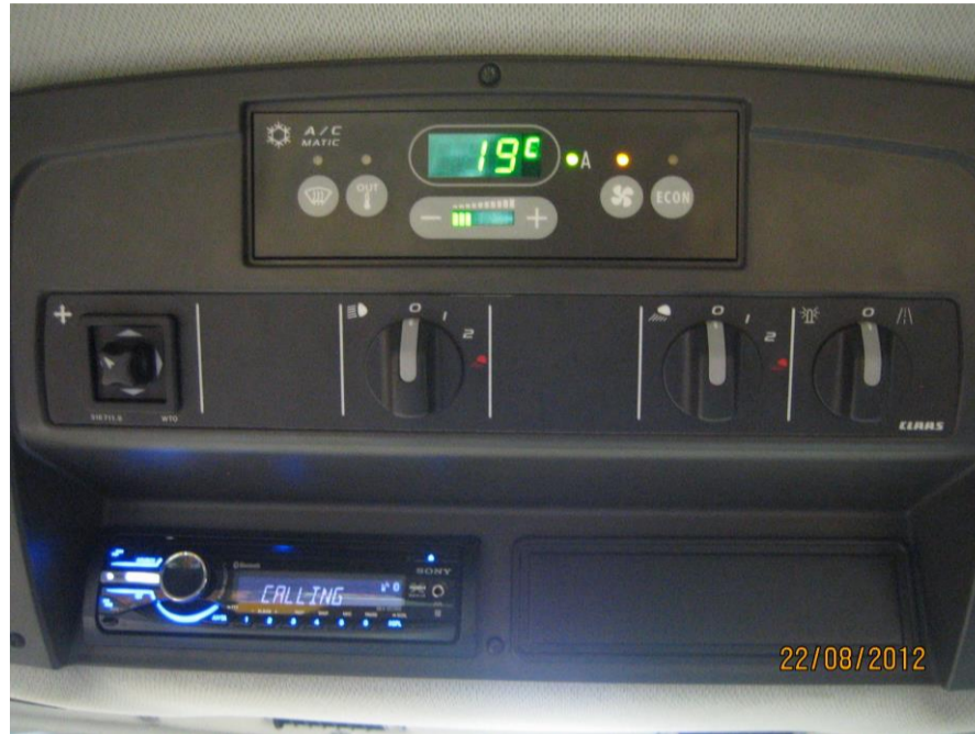
Figure 8 Showing The Lighting And Air Conditioning Control Panel
