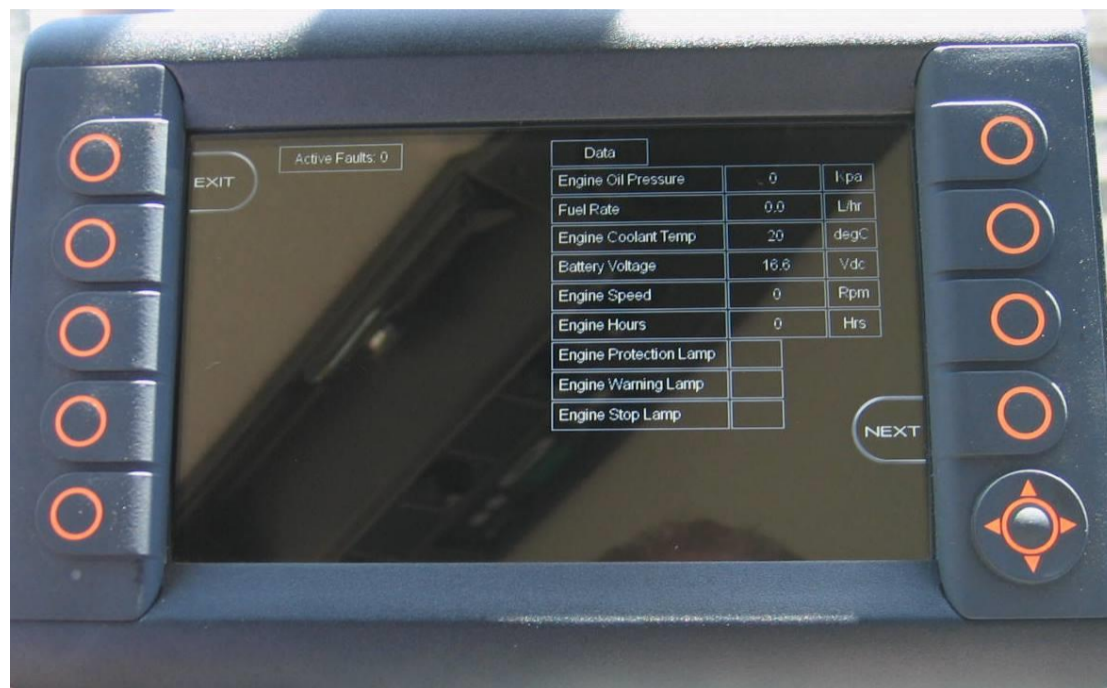
Figure 7 Showing The Engine Diagnostic Screen
